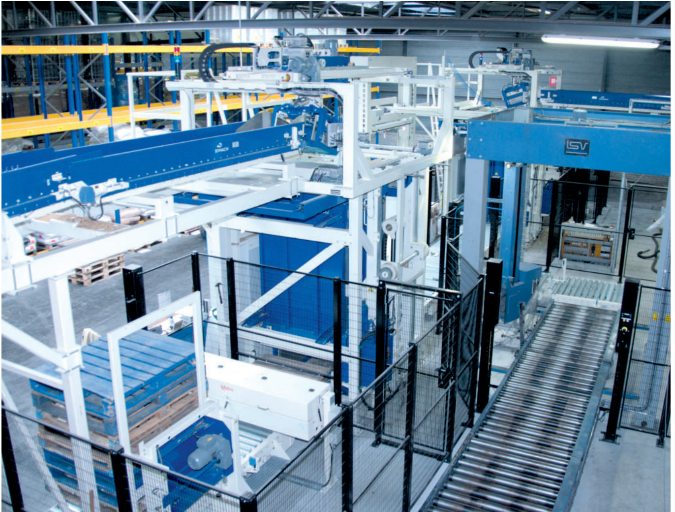
Palletizing machine with decently controlled asynchronous drive systems
