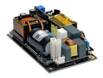
Figure 2: The GaN based technology MEP-600A supports up to 600 W output power in a wide operating temperature range (Source: Delta Electronics)
