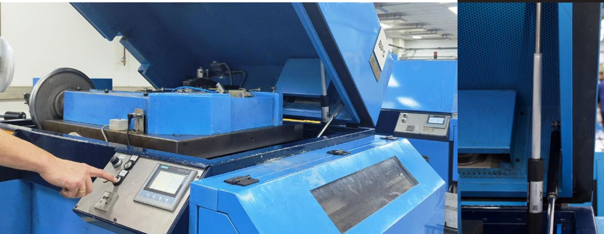
One of KeyTec Netherlands B.V.'s machine rooms in Sittard with butting machines for the production of metal pins for battery production
