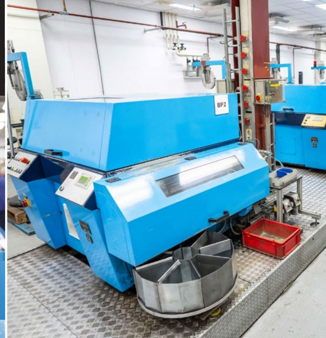
One of KeyTec Netherlands B.V.'s machine rooms in Sittard with butting machines for the production of metal pins for battery production
